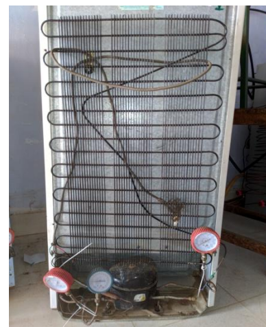
Fig 1 Proposed System with condenser coil length
