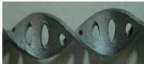
Fig. 2 Perforated twisted tape
