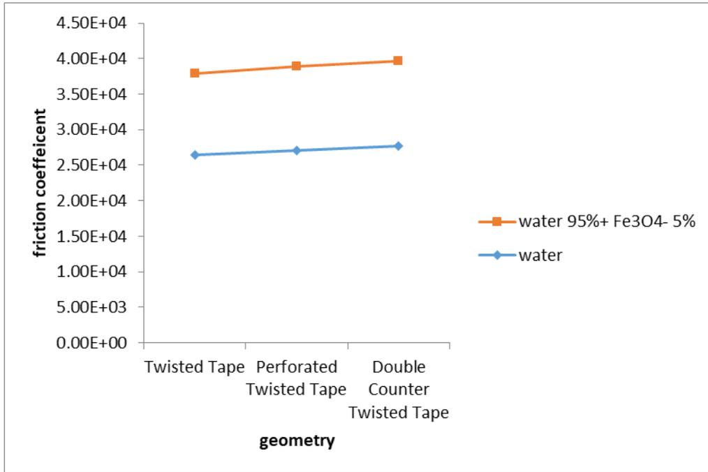
Fig 20. Friction factor in Nanofluid
