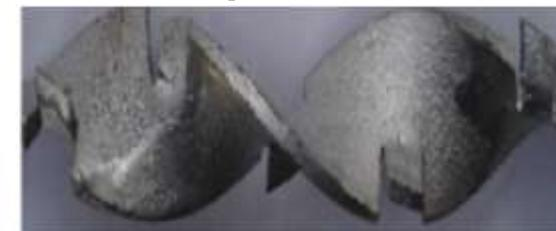
Fig 4 Jagged twisted tape
