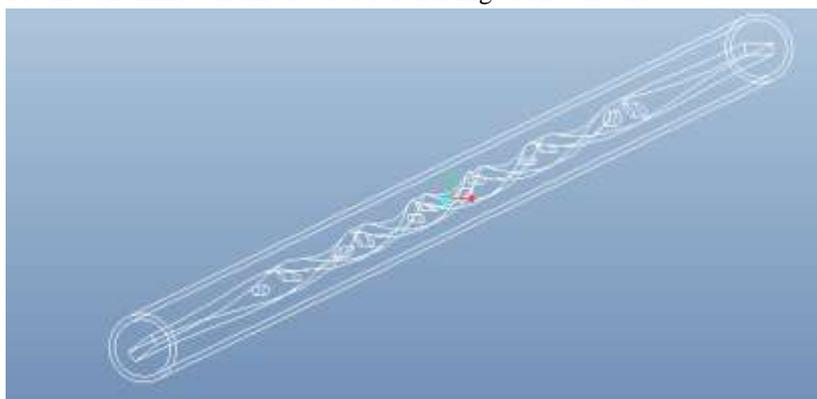
Fig. 6 Perforated twisted tapes in Pipe
