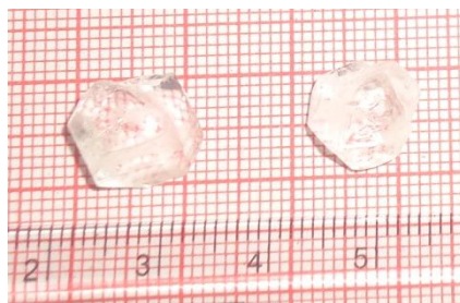
Fig. 1. Photograph of undoped and 1 mol% L_asparagine doped TGS
