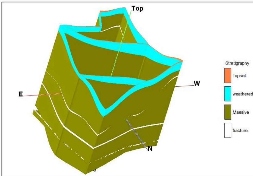
**Fig.7. 3D aquifer cross section**
