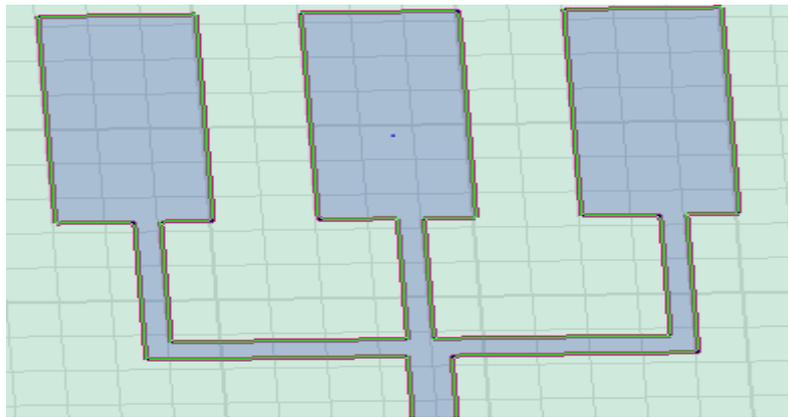
Figure (3): Rectangular Micro strip Patch Array Antenna Design.
