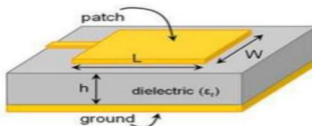
Figure (1): Structures of Micro strip patch Antenna.
