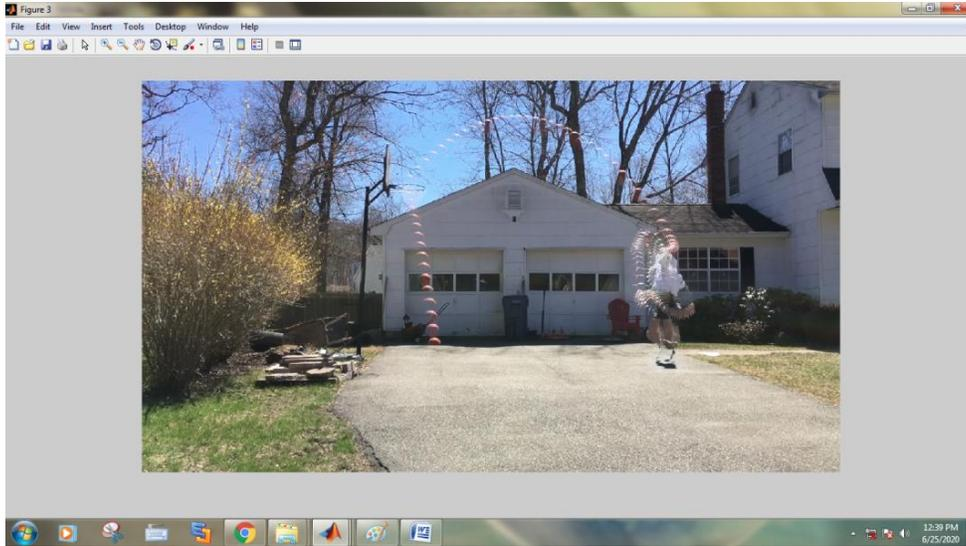
Figure 5: Object tracking and trajectory using kalman filtering
