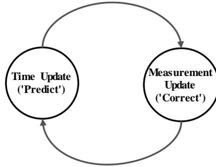
Figure 1: Basic operation of the Kalman filter
