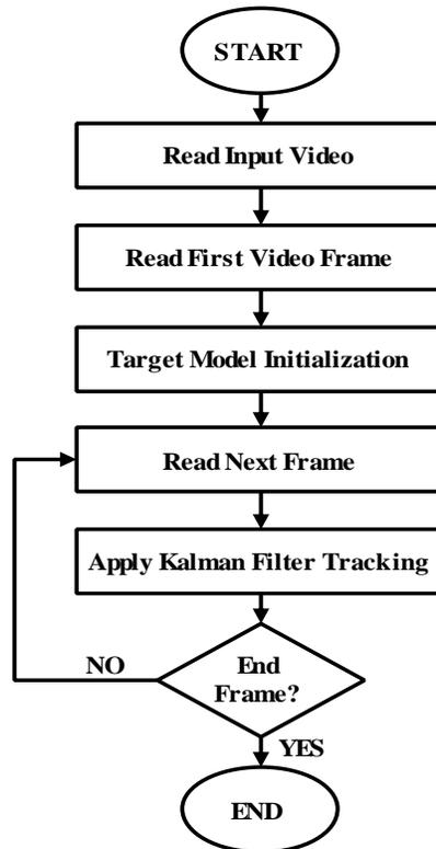
Figure 2: flow chart for kalman filter tracking
