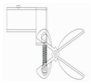
Making a device by rechargeable battery which is used to cut paper and cloth by using very basic components like motor ,battery, scissor etc.
