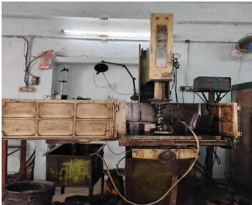
Fig 5: Die sink EDM machine
