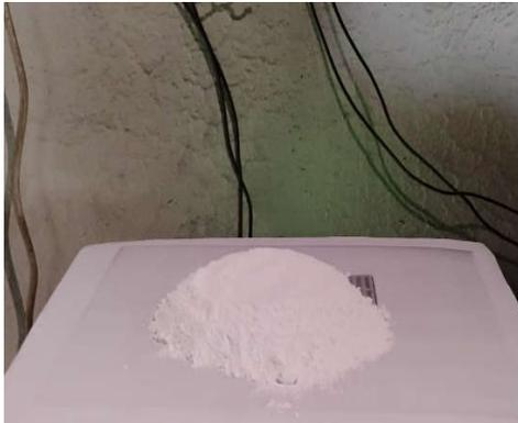
Fig 1: Boron Nitride Micro powder
