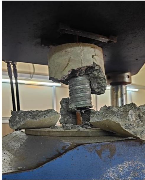
Figure. 9 Failure of surrounded concrete in (UTM)
